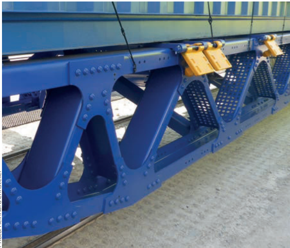
The middle part of the lightweight underframe has a steel truss structure composed of standard lorry chassis components and connected to the welded end underframes by lockbolts.
